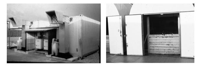
Figure1: Type 1 (left) and Type 2 (right) controlled composting bulk tunnels
